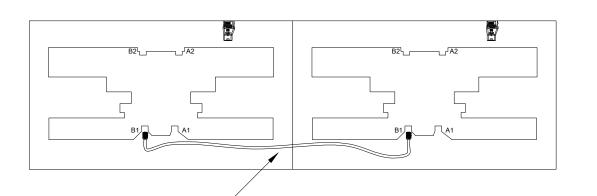
\*\*\*NOTE: THIS ROUTING IS NOT FEASIBLE DUE TO LIMITED SPACE AT THIS POINT OF THE CABINET.
