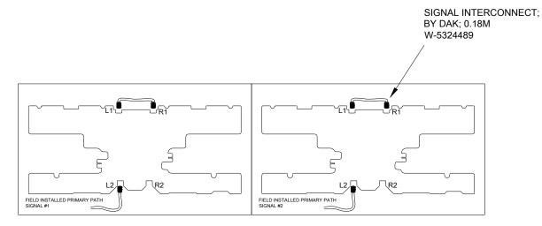
\*\*\*NOTE: ONE CAT5E/6 CABLE CAN LOAD ONLY ONE NPN-4600-0.7 CABINET WHICH HAS TWO RECEIVER CARDS. USE HORIZONTAL JUMPER ON THE HUB BOARD FOR INTERCONNECTION.
